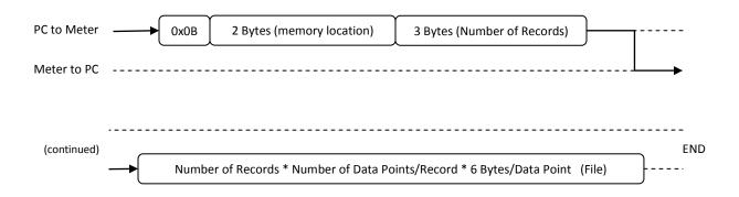
The output data is unbroken by any meter host handshaking and can be converted exactly as illustrated in the STREAM\_DATA section.
