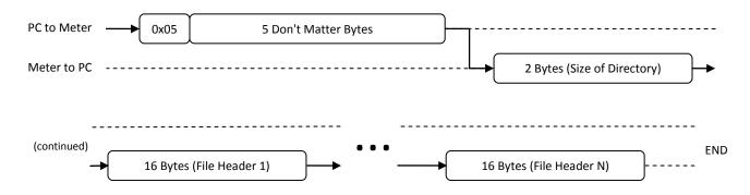
The data output of the FILE\_DIRECTORY command is a binary formatted list of file headers. The format of each directory entry (file header) will include all pertinent details to describe each file so that host software can appropriately handle file downloads.
