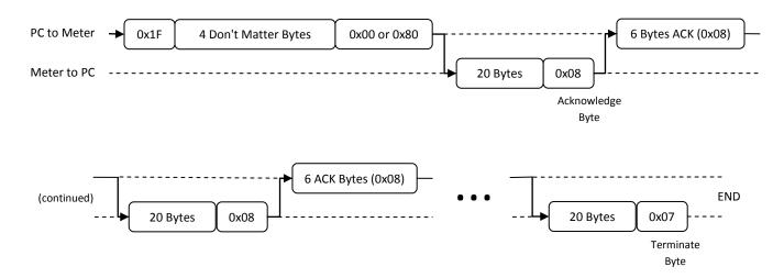
The output of this command will be in ASCII format and can be separated however the designer deems fit. The method should be selected to best suit the design but commas should separate wiper values and vertical bars should be used to separate digital pots, different ADC settings, etc. The final 20 byte block may have filler bytes in it to round out the total transmission. These filler bytes should be semi-colons.
