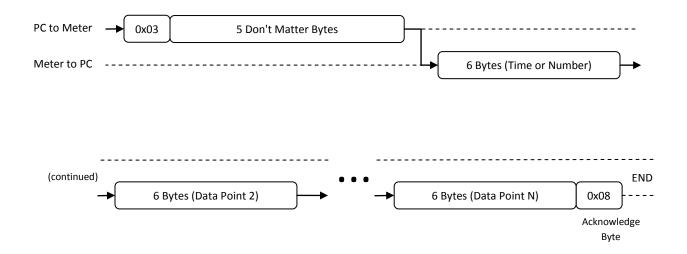
The output from STREAM\_DATA has already been described as a block of bytes equal to the number of data points multiplied by six plus an acknowledge byte however each six byte data point must be further parsed to provide usable data. Six bytes is equal to 48 bits: the first 12 are used for configuration information, the next 4 are used for sign and decimal information, and the final 32 bits are the actual number.
