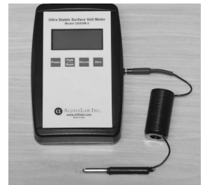
Meter Ground Wire
