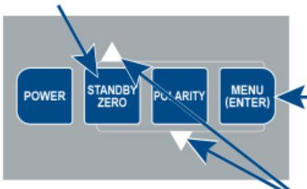
⑨ Other settings are found by pressing 'Menu(Enter)' for zero, data, and display and to see system information. To navigate in the menu, use the 'Standby Zero' and 'Polarity' buttons (white up/down arrows).
