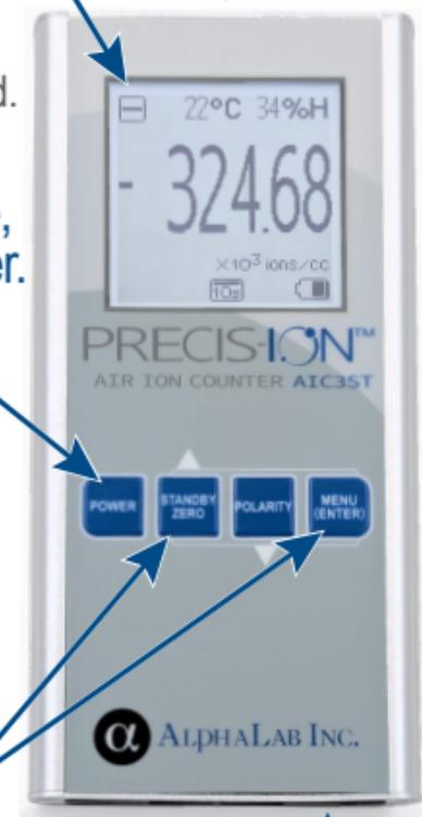
⑤ There may be an offset present in the readings that should be 'zeroed'. To zero the meter, press 'Standby Zero' and note that 'Rezero' is automatically selected. Press 'Menu(Enter)' to zero and wait for the animation to count down. Press 'Standby Zero' again to exit and begin measuring.
